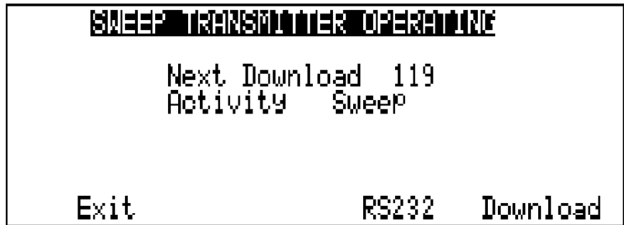
Figure 5-29 Forward Sweep Transmit Screen
